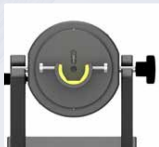
Step 5 Pull out the locating pin on the left hand side of the stand. Rotate the PET Pot 90° towards you so you can view the bleed needle hole. Insert the bleed needle through the hole and into the vial. Carefully bend the bleed needle away
