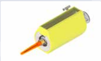
Step 7 Insert a syringe with a sheathed needle into the syringe shield.
